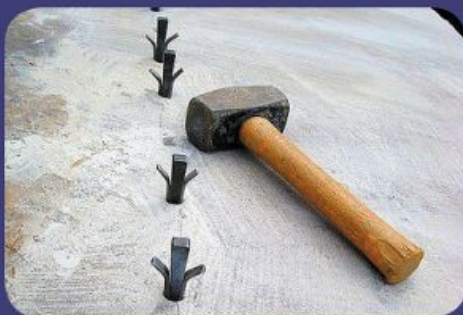
▲ Plug and feather extraction, note the fracture running between the plug and feathers.
