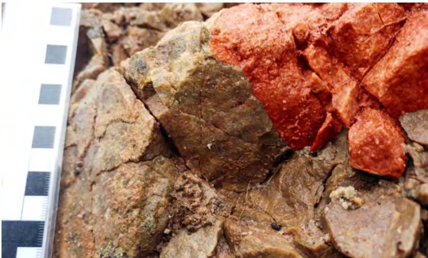
Figure 10 – The scale bar rests on a bedding plane. The fissure infill on the right has been coloured to emphasize the nature of the junction with the quartzite where it cuts across the bedding.
